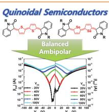
Quinoidal organic semiconductors containing dichalcogenophene (quinoidal bithiophene and quinoidal biselenophene) are designed and synthesized by facile synthetic route. Due to the extended delocalization of quinoid structure, they show low band gap and amphoteric redox behavior. Compared with common aromatic compounds, such unusual properties of quinoid structure give rise to balanced ambipolar charge transport in the top gate field-effect transistor devices.
