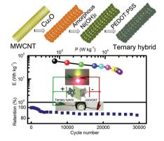
Ternary hybrid: A ternary hybrid material comprising of amorphous Ni(OH)<sub>2</sub> deposited on multiwalled carbon nanotubes wrapped with conductive polymer exhibits an ultrahigh gravimetric specific capacitance of 3262 F g<sup>-1</sup>. The assembled asymmetric supercapacitors exhibit a high specific energy density of 58.5 W h kg<sup>-1</sup> as well as excellent long cycle life (86% capacitance retention after 30 000 cycles).
