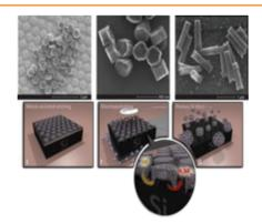
The fabrication of disc-shaped porous silicon nanoparticles through nanosphere lithography and metal-assisted chemical etching is described. The presented method provides a facile approach to controlling the shape and size of the resulting porous silicon nanoparticles. The targeted delivery of an anticancer drug to cancer cells is undertaken to demonstrate the potential of these particles as drug nanocarriers.
