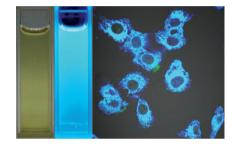
A facile, low cost, and versatile way to prepare monolayer MoS<sub>2</sub>/WS<sub>2</sub> quantum dots on a large scale with fluorescent properties is proposed via the combination of sonication and solvothermal treatment of MoS<sub>2</sub>/WS<sub>2</sub> powder. The prepared MoS<sub>2</sub>/WS<sub>2</sub> quantum dots exhibit low cytotoxicity and good cell permeability in living cells as well as excellent electrocatalytic activity toward hydrogen evolution reaction.
